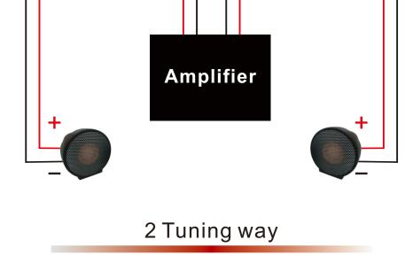
After connect well the mid-tweets with your amplfier,ac--cording to original car speaker sound, if original car loss tweeters,increase the HPF of this set of mid-tweets,make up for the lack of tweeter of the original car. On the other hand,if Middle is not enough,decrease the HPF of this set of mid-tweets.
