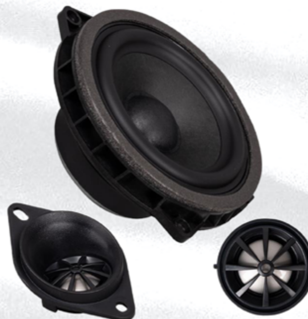
XQ-45C BMW FRONT SET 4.5" 2-WAY COMPONENT SET 30WRMS POWER / 60W MAX POWER 85dB SENSITIVITY 100-12KHz FREQ. RESPONSE 4 OHM IMPEDANCE
