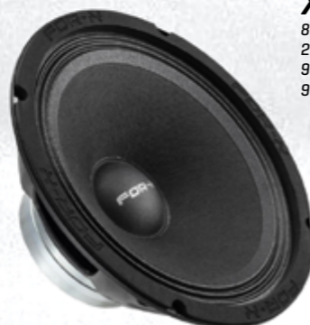
XMD-208 8" (20CM) MIDRANGE SPEAKER 200W RMS POWER / 400W MAX POWER 97dB SENSITIVITY 85-9.5K Hz FREQ. RESPONSE
