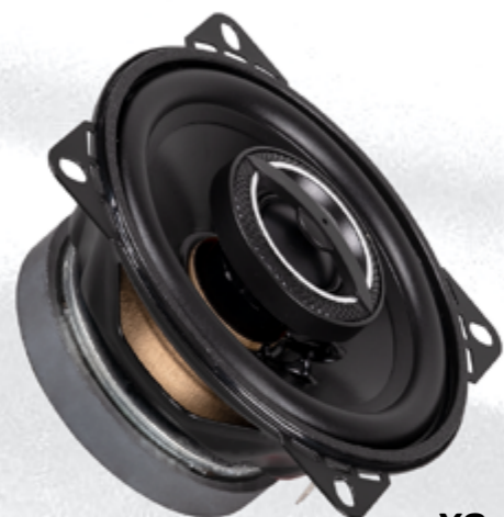
XC-310 RMS Power: 35W MAX Power: 105W Freq. Response: 100-20KHz Sensitivity: 86dB/W/M Magnet: 5.3oz Woofer: Injection Cone Midrange TW: 20mm PEI Dome
