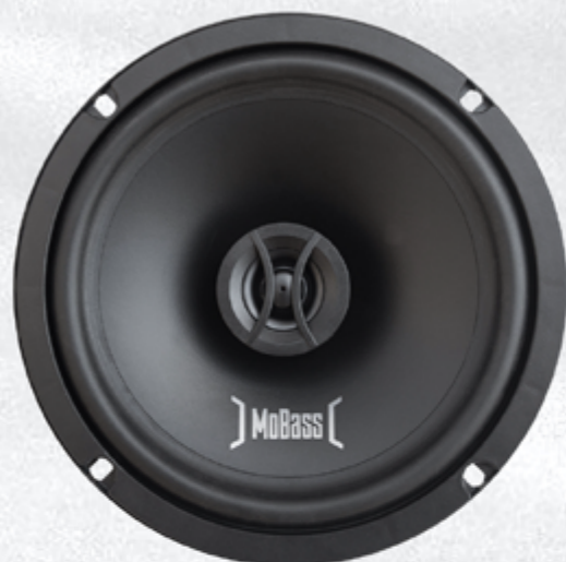
MBC-16 6.5" (16CM) COAXIAL SPEAKER 50W RMS POWER / 100W MAX POWER 88dB SENSITIVITY 88-20K Hz FREQ. RESPONSE 4 OHM IMPEDANCE
